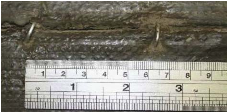
Hog-ringed CC layers opened out showing PVC surface
