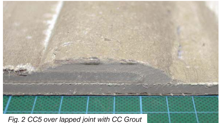
Fig. 2 CC5 over lapped joint with CC Grout
