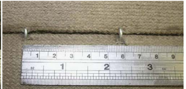
Hog-ringed CC layers opened out showing fibre surface
